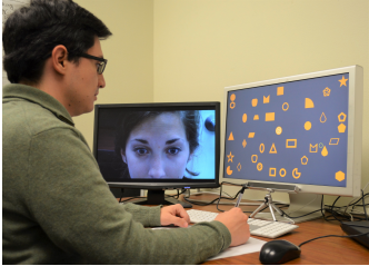
Figure 9: Video Analysis Attack: A user is trying to guess the gaze password with the help of a video and authentication interface.
