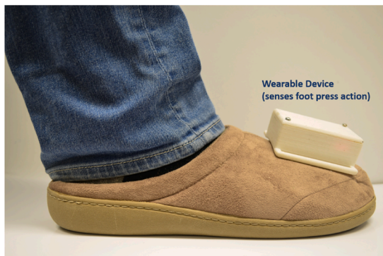
(a) Footwear augmented with pressure sensor
