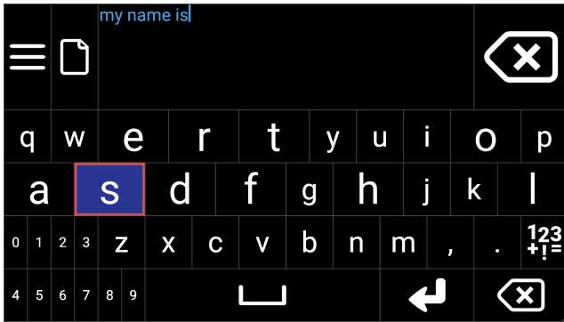
Figure 2: Customized Virtual Keyboard - High Frequency Alphabets and Functional Keys are Larger
